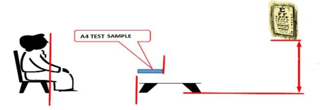
**Colour matching and surface texture:** A slight deviation of colour and / or surface texture according to Rating4 EN14323 between the test sample and Kastamonu reference sample.
